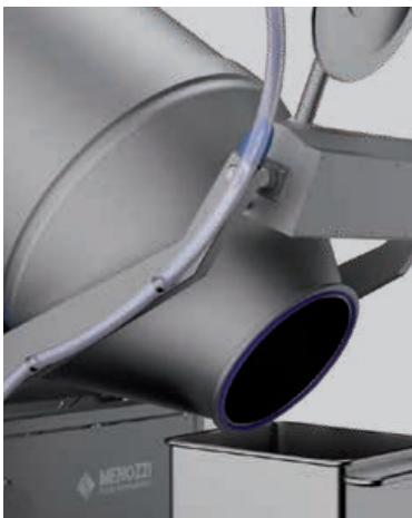
Automatic discharging program, 8 discharging steps
