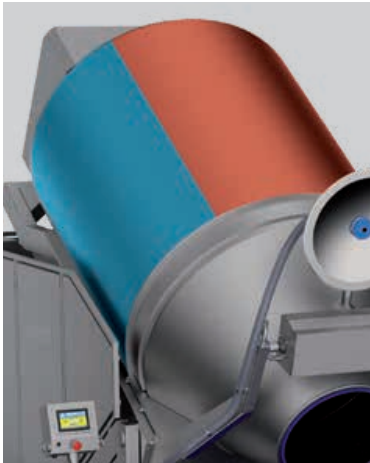
Refrigerated-heated jacketing with automatic thermal control
