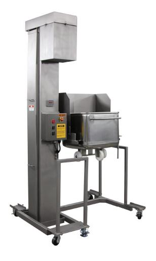
The Column Loader is an innovative solution designed to enhance efficiency and safety in food processing environments. This equipment is specifically engineered to handle standard 400lb and 600lb VEMAG carts, offering a hygienic and ergonomically friendly method for dumping contents. Its design prioritizes the health and safety of operators by reducing manual lifting and handling, which can lead to strain or injury.
