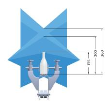
The optimized beam geometry ensures the best contaminant detection results achieved in the bottom part of the container.
