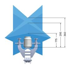
The optimized beam geometry ensures the best contaminant detection results achieved in the bottom part of the container.
